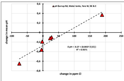
**Figure 7.** Plot of  $\Delta\text{pH}$  between yearly median data vs. the change in seasonal salt levels ( $\delta[\text{Cl}]$ ) for 2019 compared with 2018 and 2017
