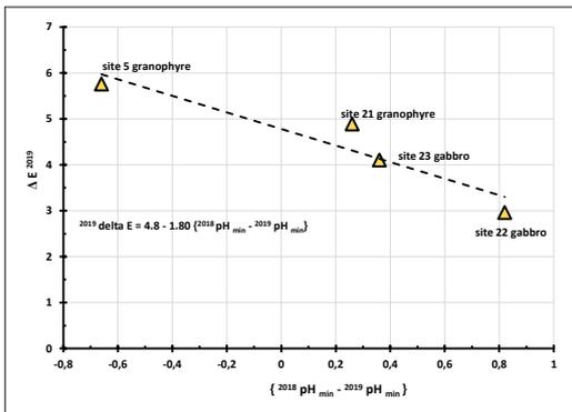
**Figure 8.** Plot of median  $\Delta E_{2019}$  for colour contrast between background and engraved areas decreasing with increasing alkaline shift in the minimum pH between 2018 and 2019
