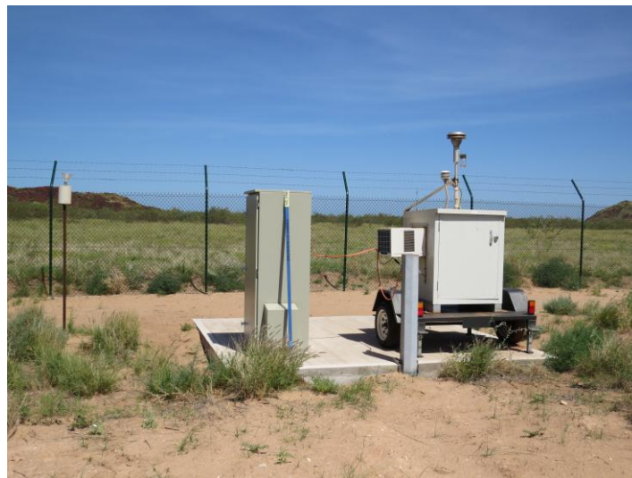
Figure 7-3 Dust deposition gauge at eastern boundary
