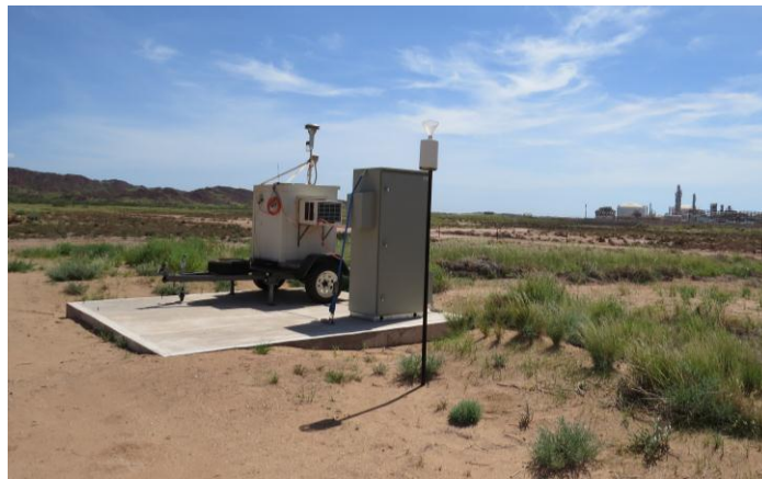
Figure 7-5 Thermoscientific TEOM 1405 (TRA2) at eastern boundary
