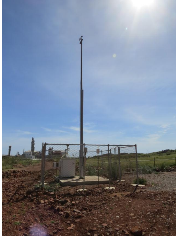
Figure 7-4 Dust deposition gauge at western boundary
