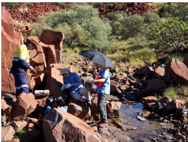
Figure 4 ASD FieldSpecPro and Konica Minolta CM-700dspectrophotometer operating on petroglyphs in the Burrup Peninsula (2013)
