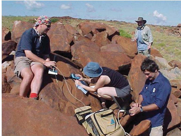
Figure 4: ASD FieldSpecPro operating on petroglyphs in the Burrup Peninsula (2005)
