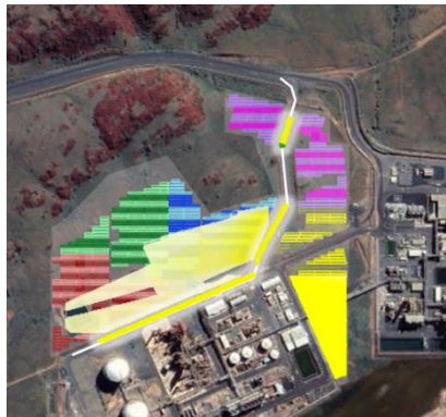
Figure 35 Yellow and green glare predicted for YPF Access 1 (clouded white) and glare source from arrays 1 and 3 superimposed on satellite image
