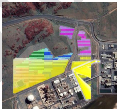
Figure 36 Yellow glare predicted for YPF Access 2 (clouded white) and glare source from arrays 1, 2 and 3 superimposed on satellite image
