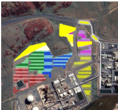
Figure 37 Yellow glare predicted for YPN Access (clouded white) and glare source from arrays 1 and 2 superimposed on satellite image
