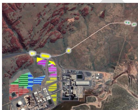
Figure 34 Yellow and green glare predicted for Village Road (clouded white) and glare source from arrays 1 and 2 superimposed on satellite image
