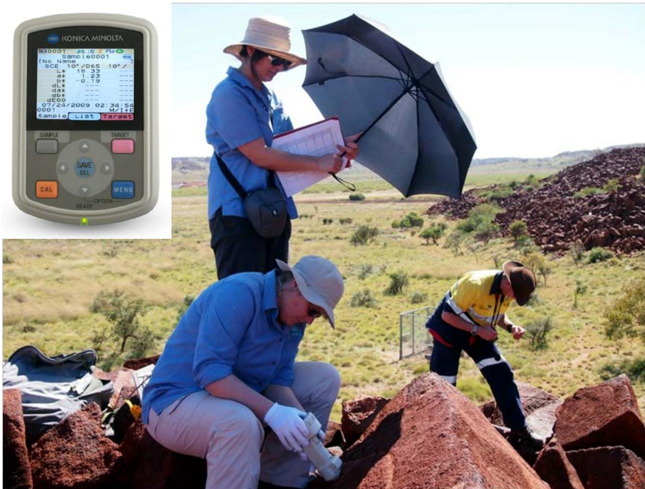
**Figure 3. Kona Minolta Photospectrometer in use for the measurement of Petroglyphs (Site 7)**
