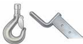
The lifting hook should have well-rounded edges
